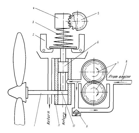
1.Passage between Governor and Airscrew 2.Weight 3.Spring 4.Toothed Rack 5.Control Shaft 6.Slide Valve 7.Oil Pump 8.Passage to Supply Oil from Engine to Governor 9.Reducing Valve 10.Slide Valve Shoulder 11.Drive Shaft
