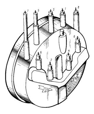
NOTE: Figures indicate numbers of cylinders to which distributor cables are to be connected. Cables from LH magneto run to front spark plugs, from RH one, to rear spark plugs. Magneto Distributor Figure 201
