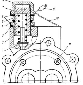
Oil Pump Reducing Valve Assembly Figure 3
