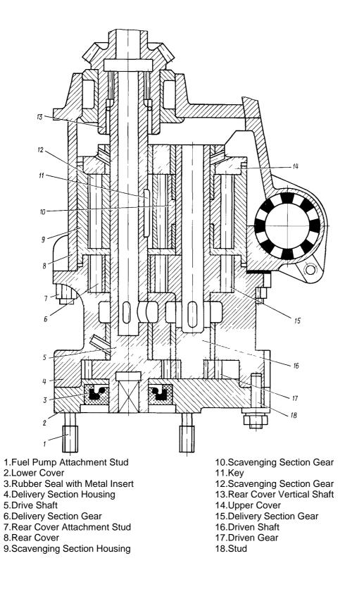
Oil Pump MN-14A. Longitudinal Section View Figure 2
