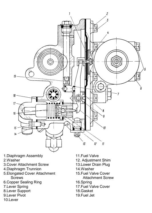
Diaphragm Assembly and Fuel Valve Figure 3
