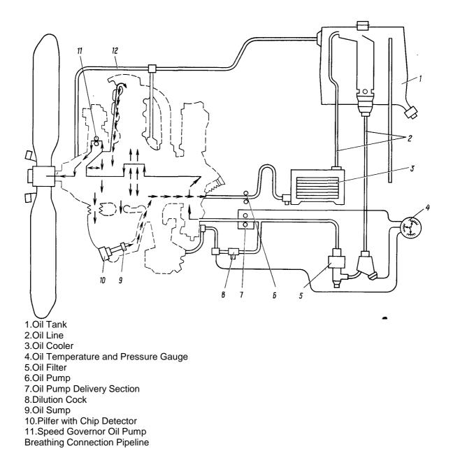
Engine Lubrication and Breathing Diagram Figure 1
