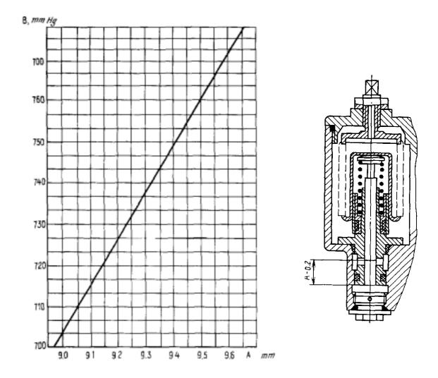
Carburetor Altitude Control Needle Position Versus Barometric Pressure (Barometric Graph)Figure 203
