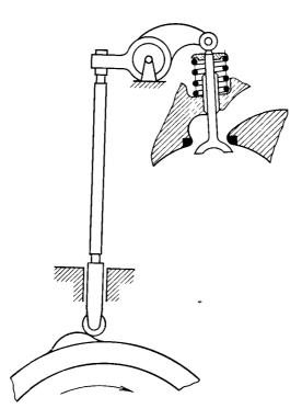
Timing Mechanism Schematic Diagram Figure 6
