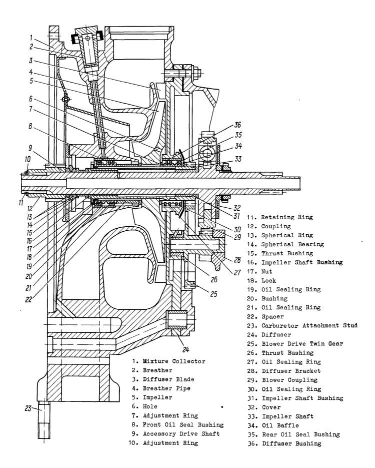
The front part of the steel bushing has drilled holes communicating with the atmosphere through the annular recess, passage in the vertical wall and a steel pipe.
