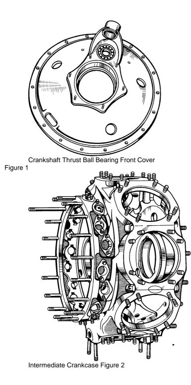
Three holes provided in the conical wall of the front cover are intended to breath internal spaces of the crankcase and a hole for draining oil from the gearbox housing to the intermediate crankcase.
