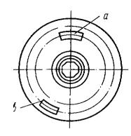
Air is fed through the port located, away from the slide valve center and through the oval holes in the distributor cover to the lower cylinders Nos 4» 5, 6 and 7 for scavenging them during exhaust stroke,
