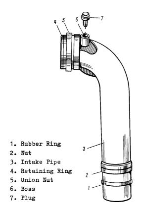
Intake Pipe of Cylinders Nos 4, 5 and. 6 Figure 4
