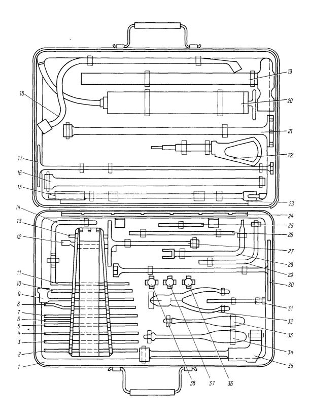
Arrangement of Airborne Tools in Case Figure 1
