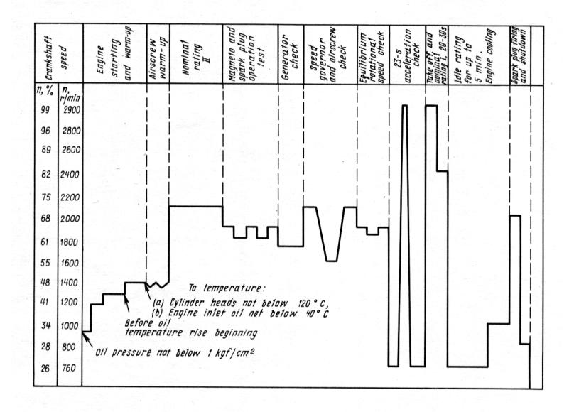
Engine M-14P Test Run Chart Figure 201
